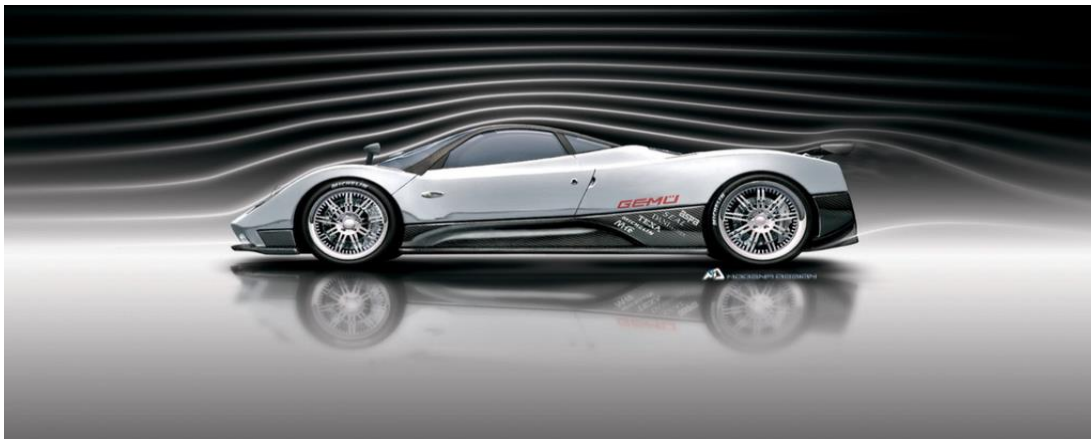
Figure 1. A car in a wind tunnel simulates a car driving down the road. Smoke is blown at high speeds to study the way the air flows over the car. The low pressure zone can be seen behind the car by noticing that the streams of smoke bend inwards at the back of the car.
